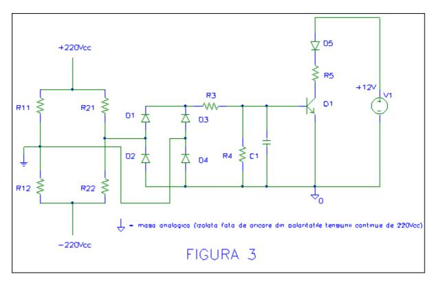
A measuring scheme with a Wheatstone bridge was selected. Two arms of the bridge,  $R_{11}$  and  $R_{12}$  respectively, are formed by the insulating resistance between the two polarities and earth, each of it paralleled with a physical resistor (500 - 1000k $\Omega$ ). The value of the other resistors in the bridge ( $R_{21}$  and  $R_{22}$ ) are chosen so that all the bridge resistors have approximately the same value at the balance point.
