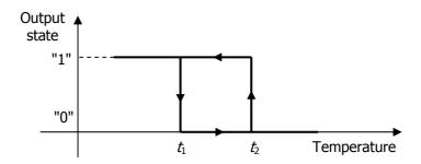
Figure 2. Programmable temperature characteristic
