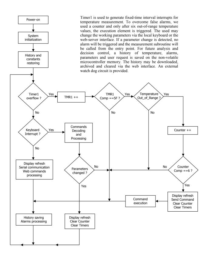
Figure 3. Software flow diagram
